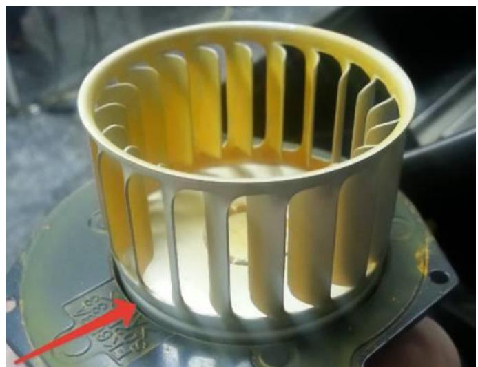
Blow out the salt from the impeller and fan surface. Fix the impeller and launch the fan in a testing mode.
