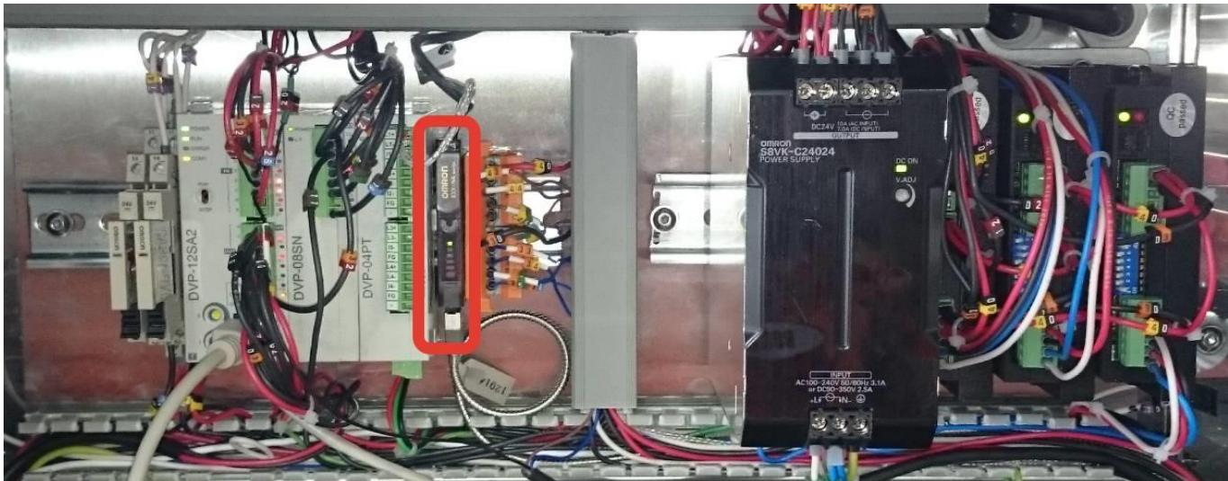
By default it is set in the middle position. Adjust it by an potentiometer.
